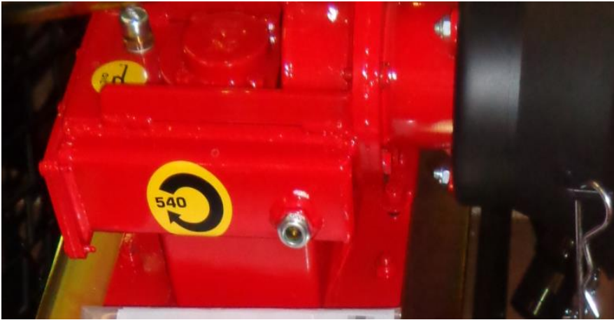
Figure 10 top gearbox with vent and sight-glass window
