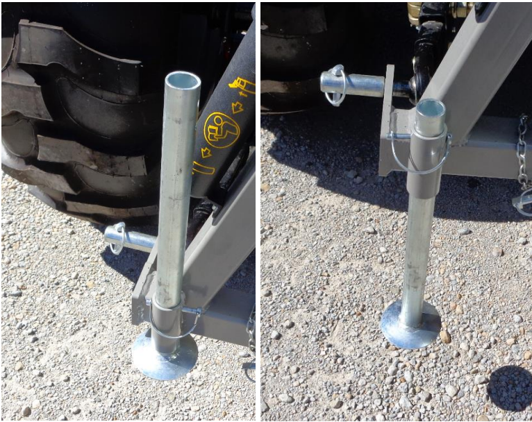
Figure 11 - jack stand shown up for mowing and transport and down to park
