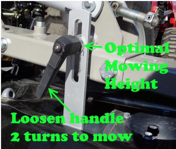
Figure 7 - three point hitch height is optimal when handle is about 60% up the slot
