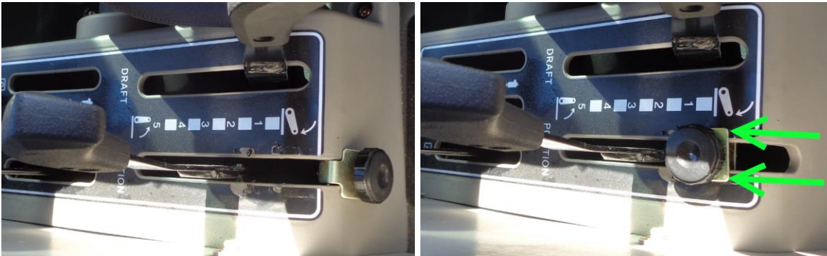
Figure 9 - Position control low limit shown before and after setting low limit
