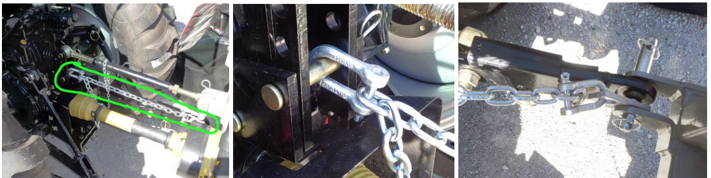
Figure 8 - low limit chain shown installed
