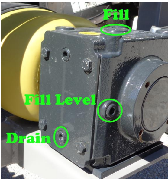
Figure 13 - 90° gearbox plug locations
