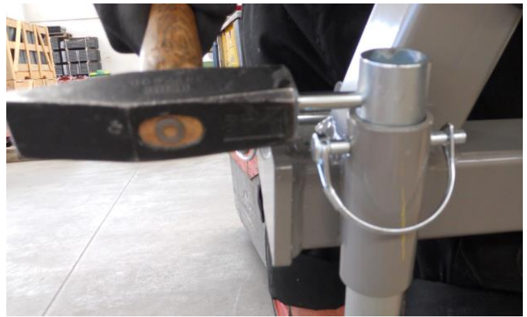
Figure 4 - drive pin into stand
