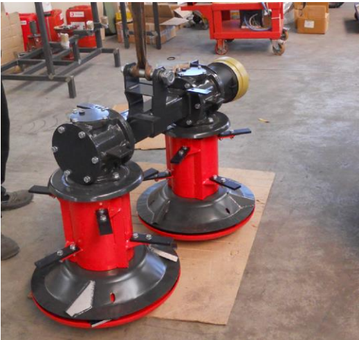
Figure 2 - drum unit on floor ready for assembly
