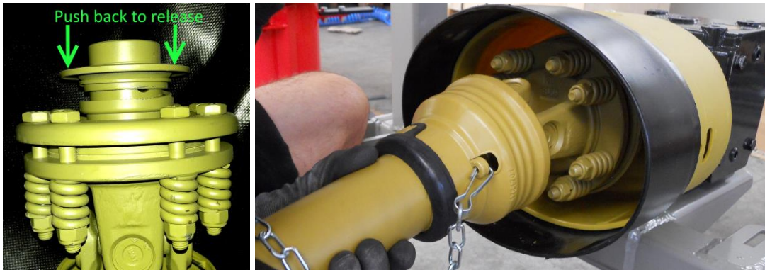
Figure 11 - install the clutch end onto the gearbox
