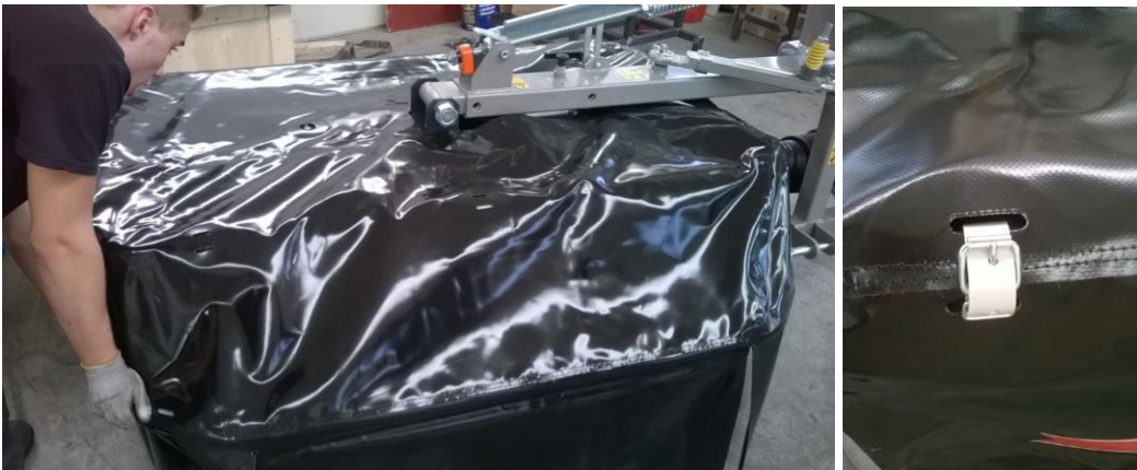
Figure 20- fit and secure the curtain over the frame
