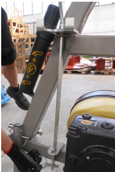
Figure 14 - blade change tool and pin with locking ring
