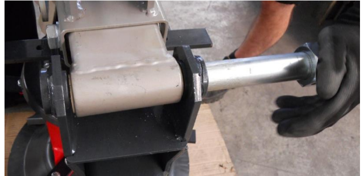
Figure 8 - align holes and push pin through
