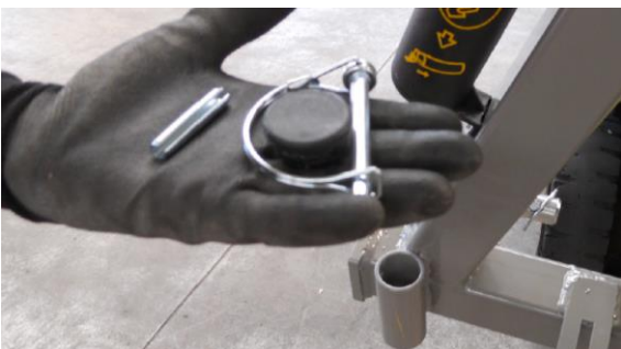
Figure 3 - remove hardware for jack stand installation
