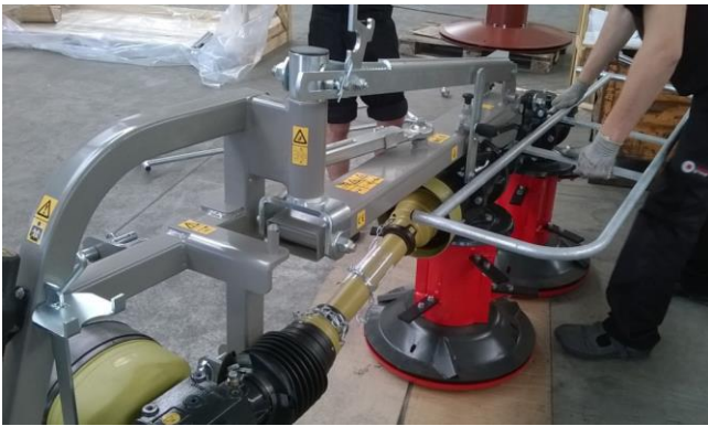
Figure 16 - attaching the rear frame
