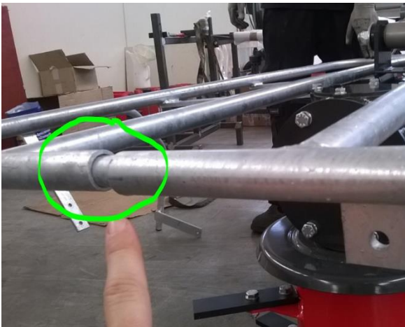
Figure 17 - alignment feature for guards
