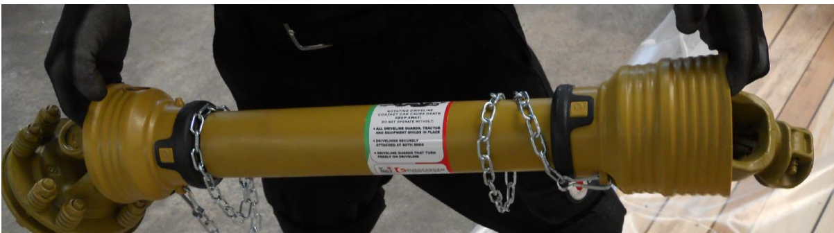
Figure 10 - driveline that goes from the tractor to the mower
