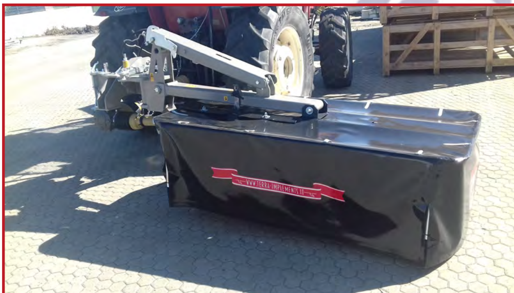
85. Sarracenia 180 Hydraulic version assembled.
