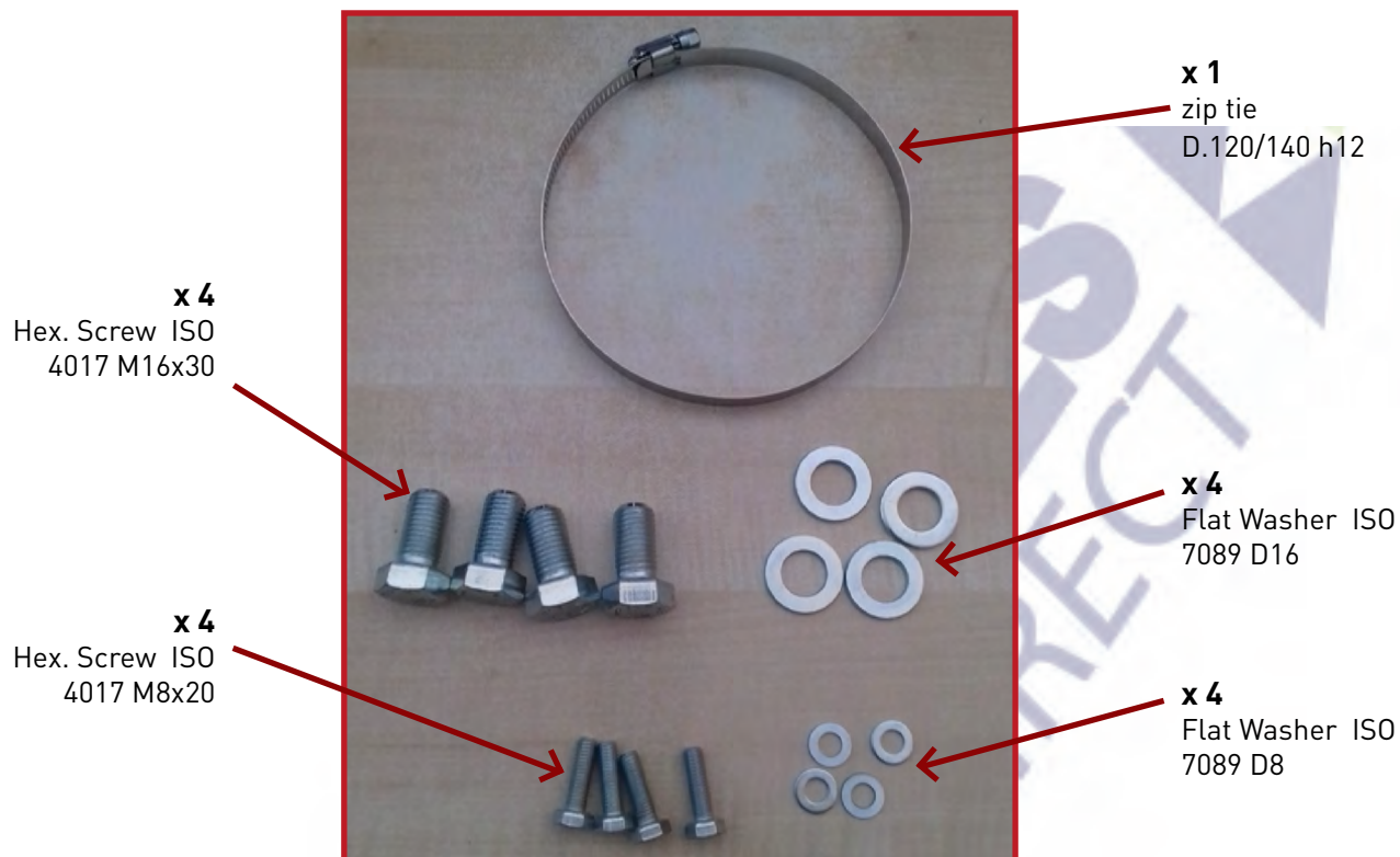
37. Screws necessary for gearbox's assembly.
