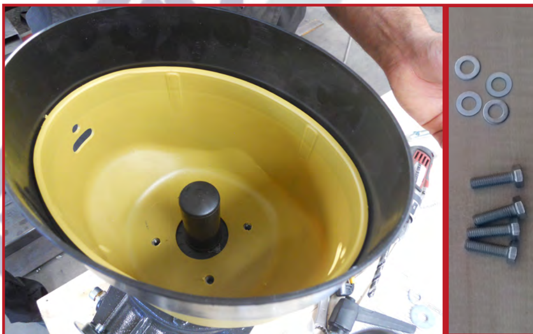
38. Take the PTO guard, position it on the gearbox and insert the washers and the screws.
