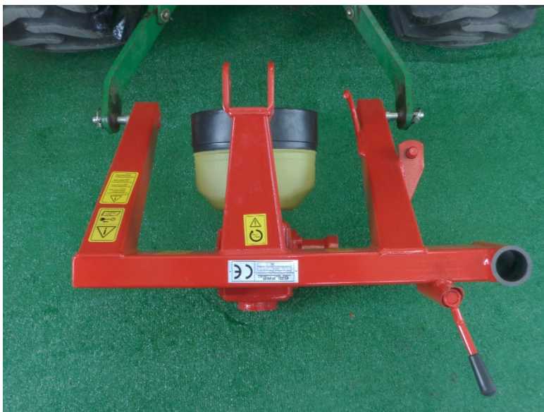
Figure 7 3 point hitch attached to tractor's lift arms
