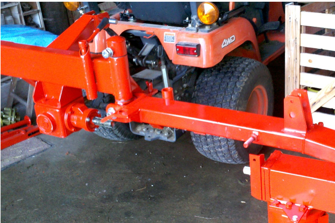
Figure 13 lower lift arm in place
