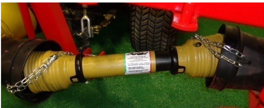
Figure 22 guard chains attached
