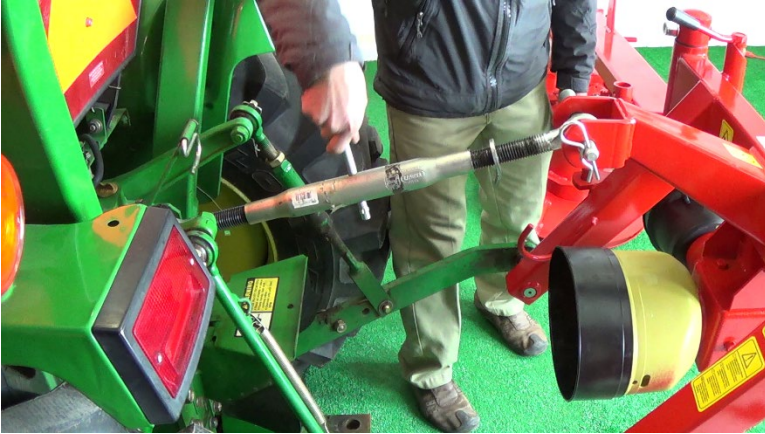
Figure 8 plumb the 3 point hitch unit using the top link
