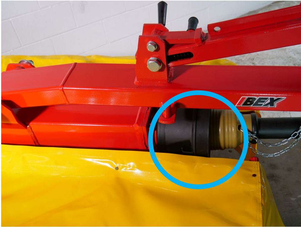
Figure 5 the other small guard installed on the drum unit
