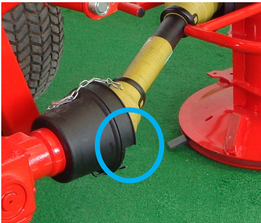
Figure 4 smaller guard with cut-out facing the rear (cutout may look different than picture)
