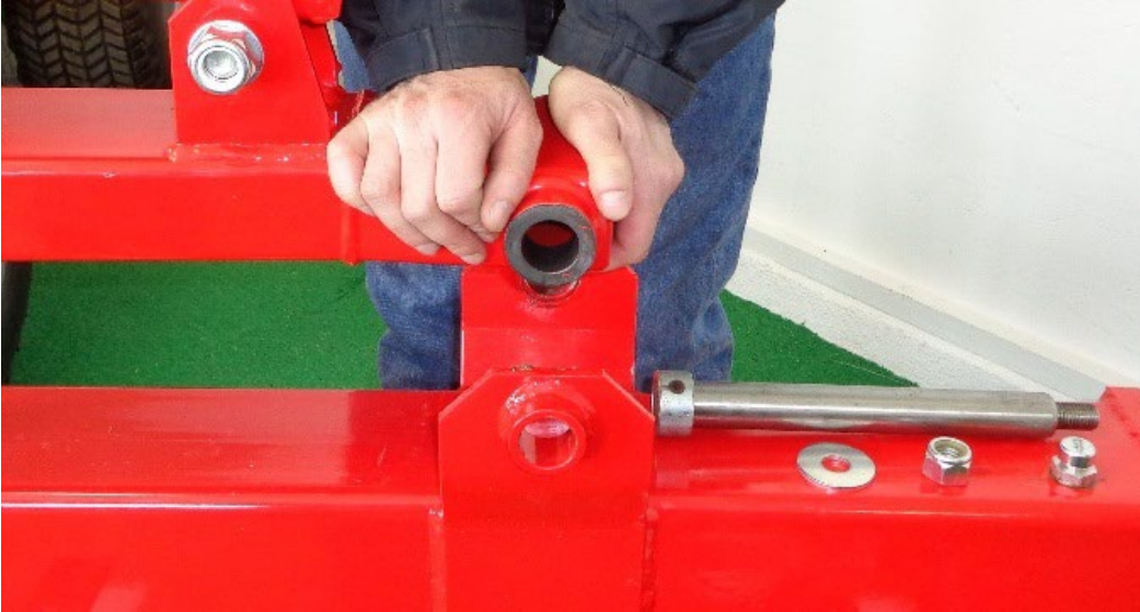
Figure 16 push the lower arm down to line up with drum unit
