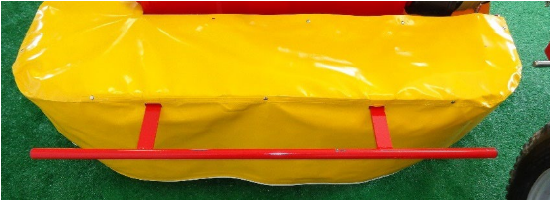
Figure 27 curtain installed with 2 holes for toe guard facing forward
