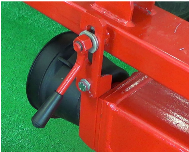
Figure 23 pivot restrictor plate & handle installation
