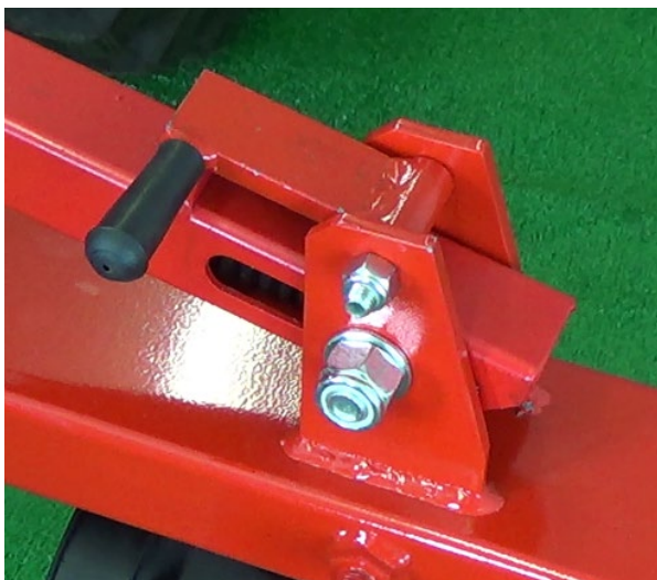
Figure 19 transport lock installed
