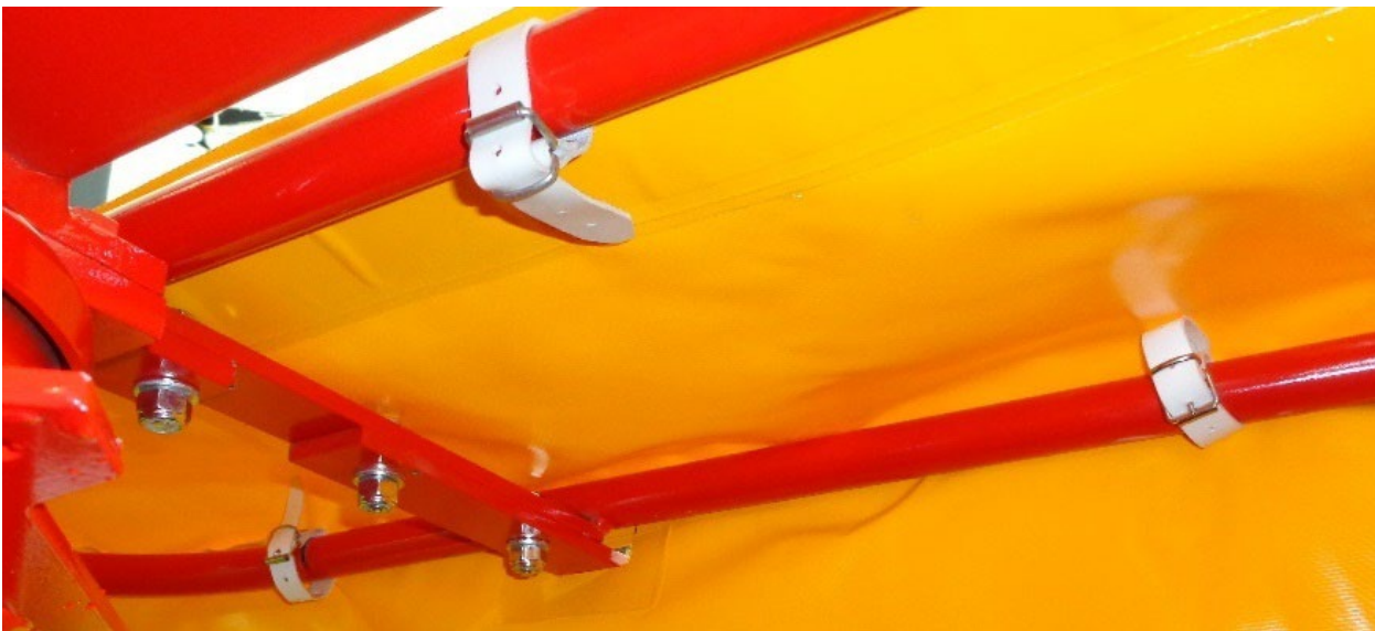
Figure 26 curtain straps secure to the guard frame
