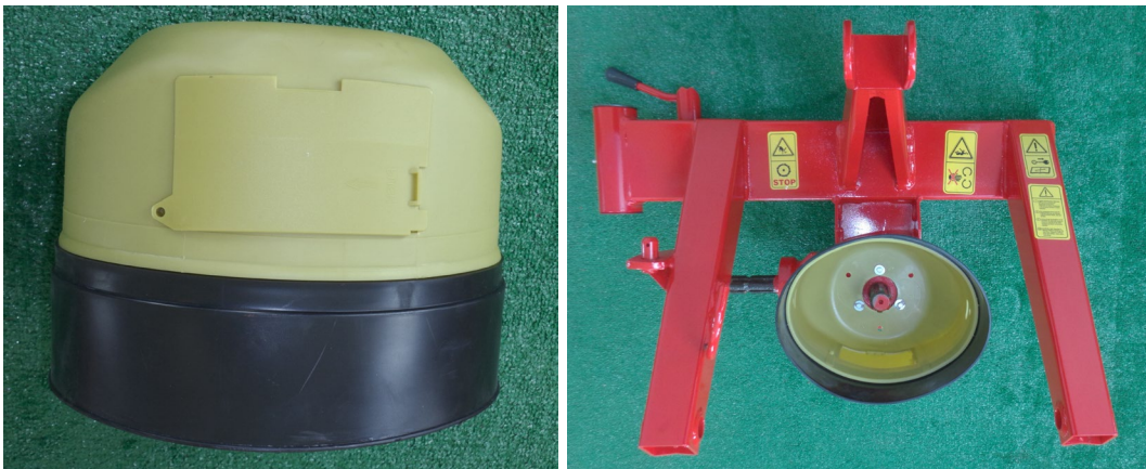
Figure 3 larger guard installed on the gearbox facing the tractor
