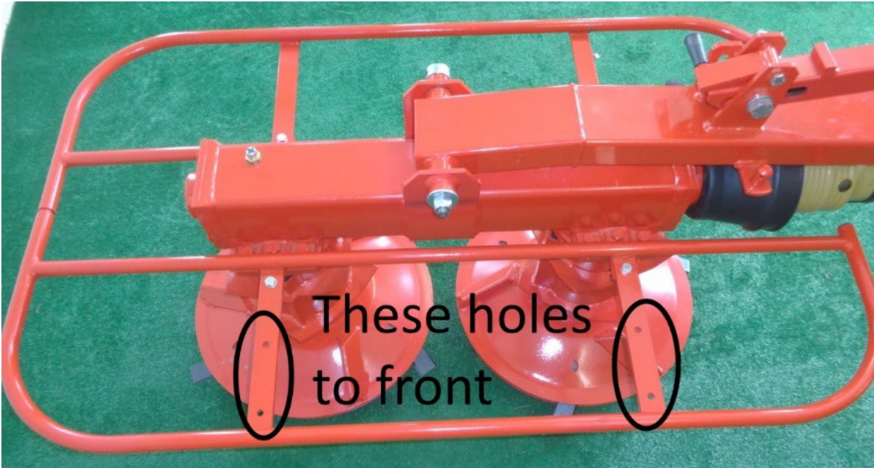
Figure 25 front guard has six holes
