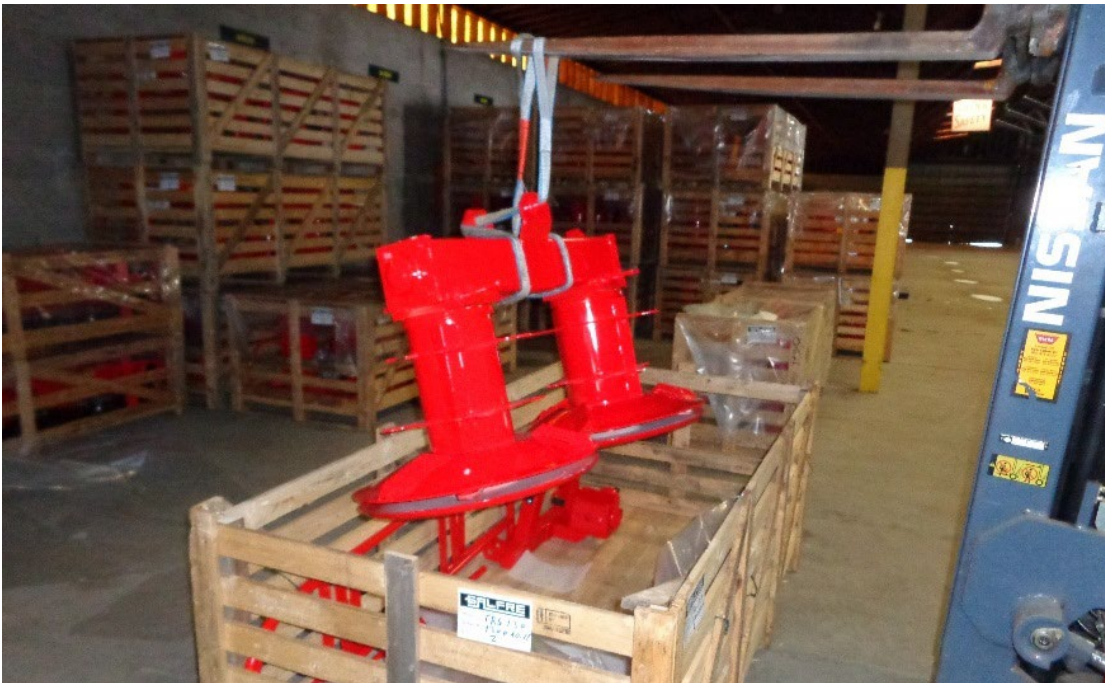
Figure 1 lifting the drum assembly
