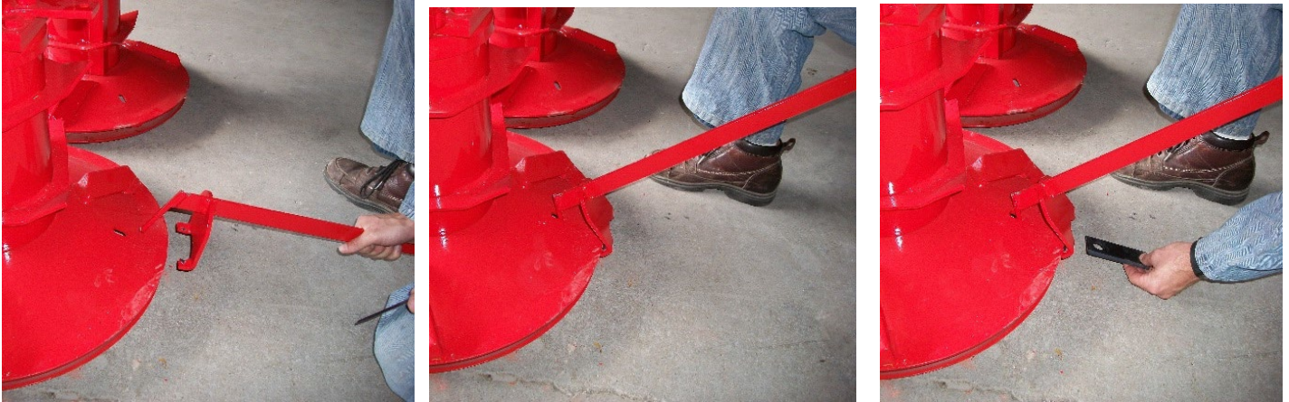
Figure 10 installing a blade
