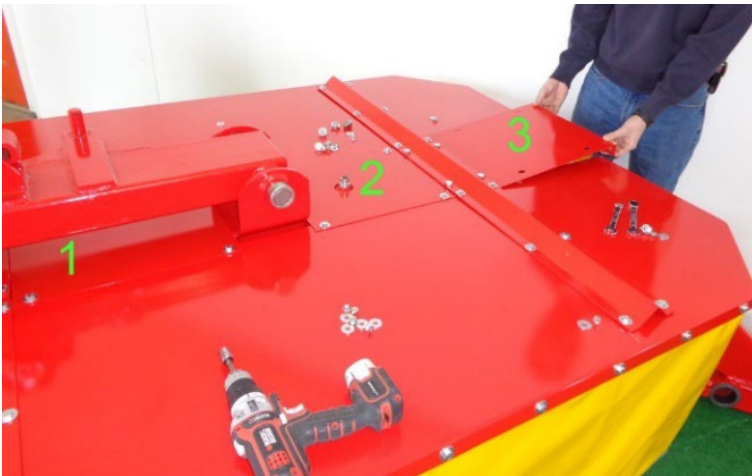
Figure 21 shield plates shown located on top of guards
