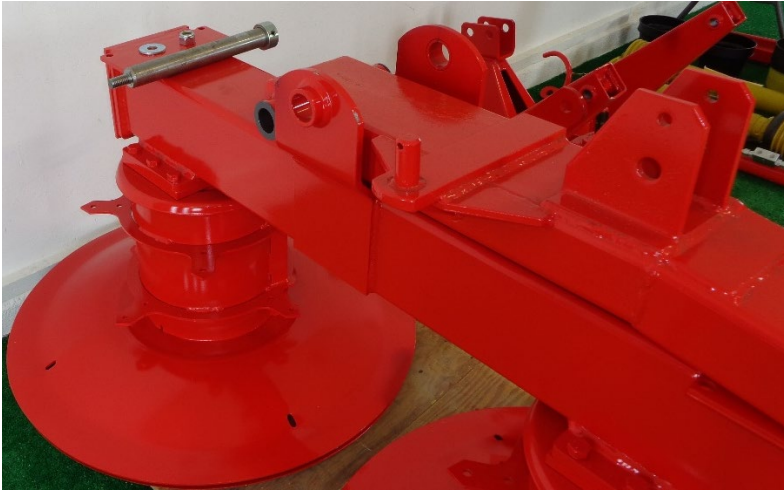
Figure 7 drum support arm before attachment
