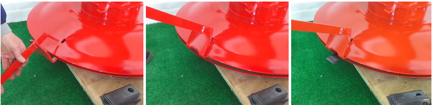
Figure 14 installing blades with the blade change tool
