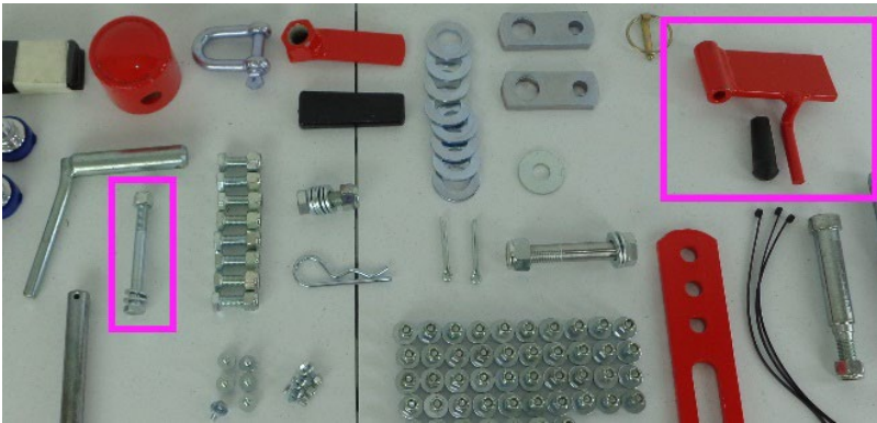
Figure 29 hardware for spring arm transport lock
