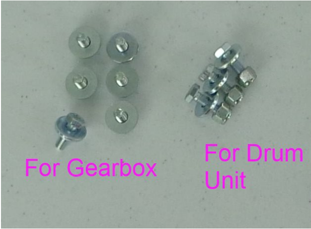
Figure 23 hardware to attach PTO guards
