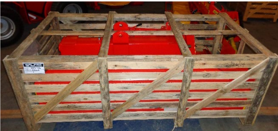
Figure 3 Drum Mower in crate as shipped
