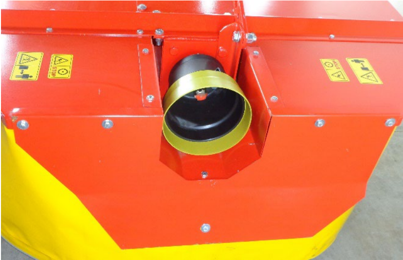
Figure 24 shields installed as well as PTO guard
