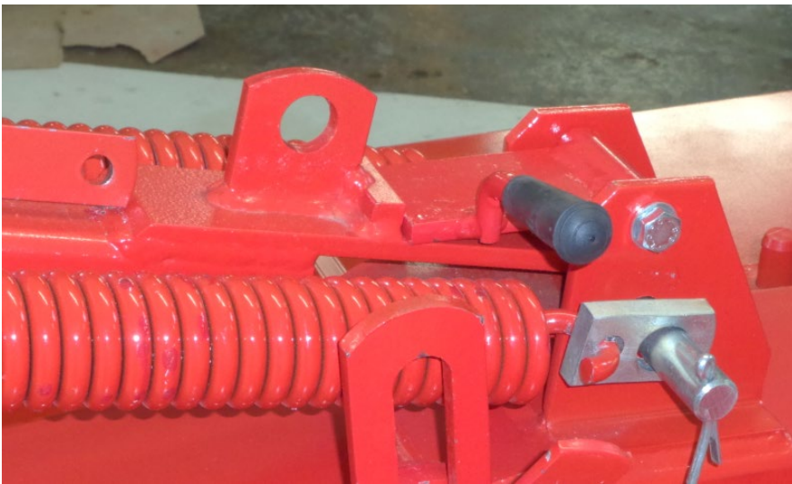
Figure 30 spring arm transport lock shown installed and in transport position
