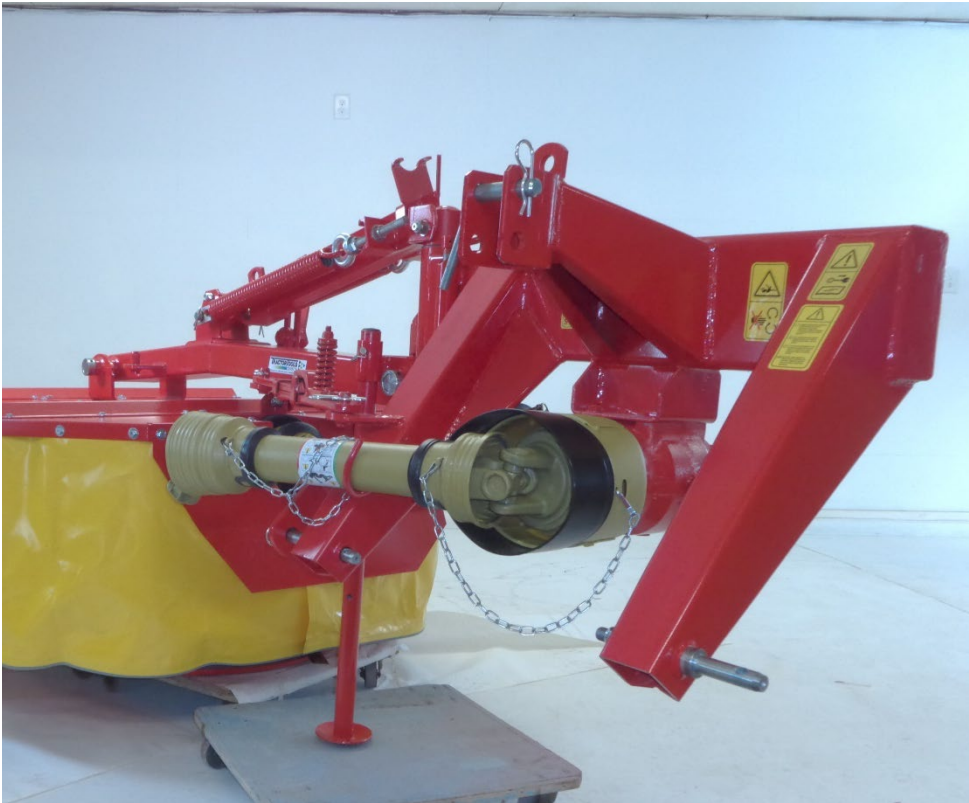
Figure 33 larger, oval-shaped guard is installed on the front of the gearbox, facing the tractor
