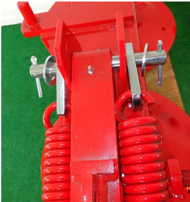
Figure 10 spring attachment hardware shown with springs
