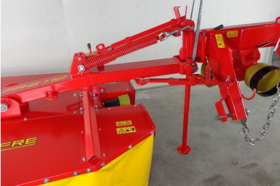
Figure 35 lift the three point assembly up and install the jack stand
