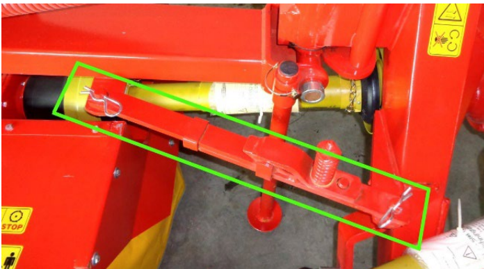
Figure 28 breakaway protection arm in mow position
