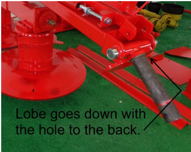
Figure 13 install pin with hole to back
