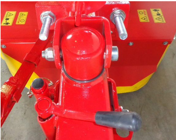
Figure 27 top cap and spring arm bolted in place
