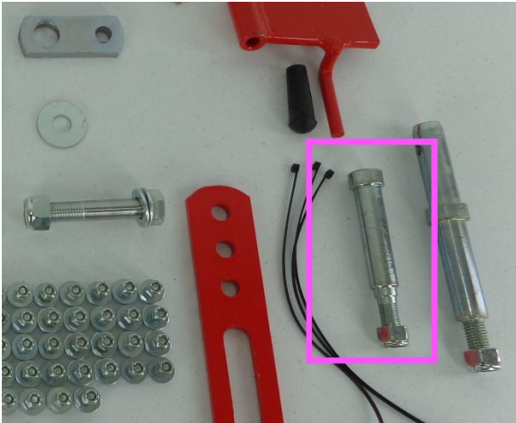
Figure 26 pin to attach spring arm through top cap
