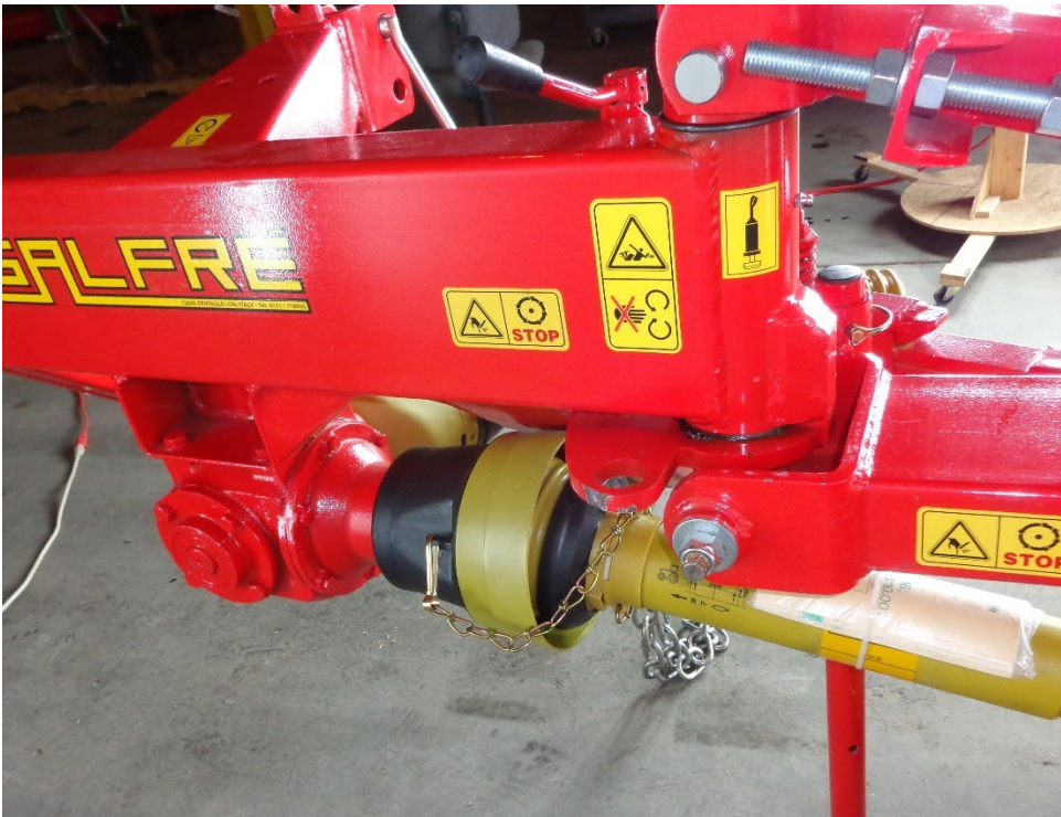
Figure 34 smaller PTO guard installed on the 90 degree gearbox, facing the drum unit
