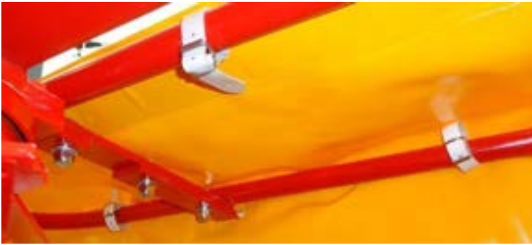
Figure 37 curtain straps secure to the guard frame
