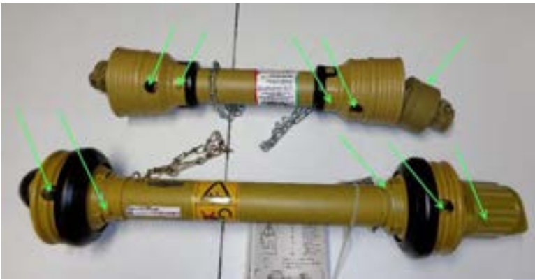
Figure 6 grease points on PTO drivelines
