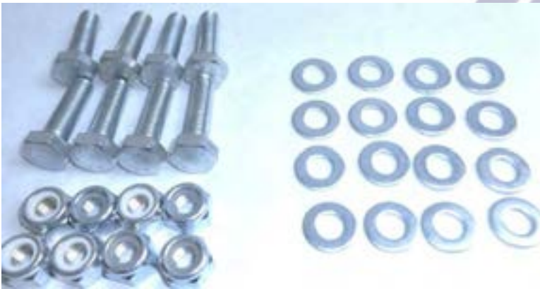
Figure 35 eight sets of fasteners used for attaching guard frame
