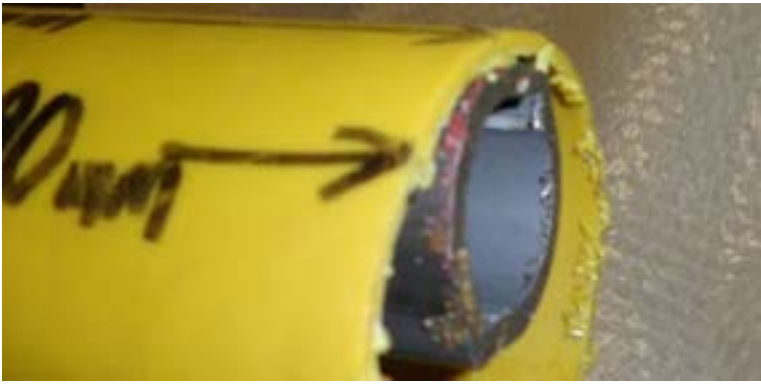
Figure 44 align end of tube to end of shaft
