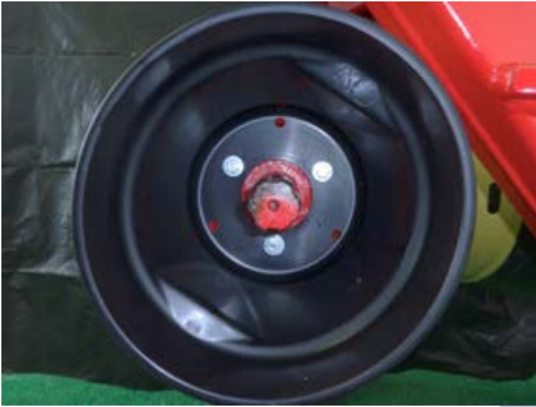
Figure 9 the third guard is installed on the gearbox
