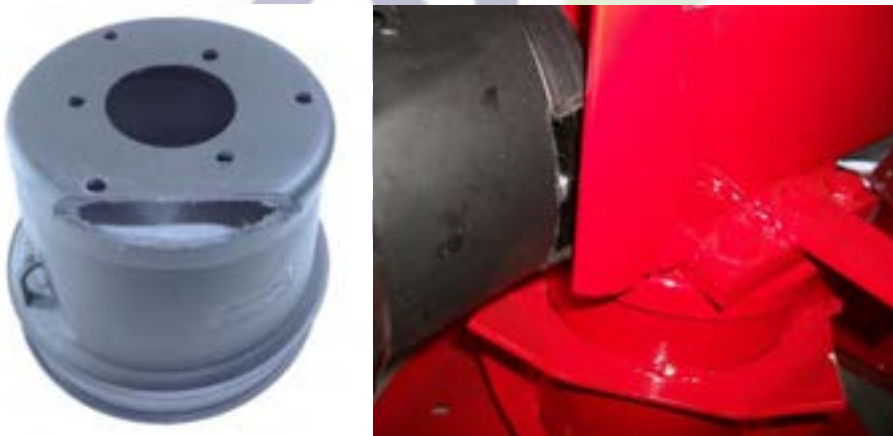
Figure 8 the guard with the notched out area is installed on the drum unit as shown
