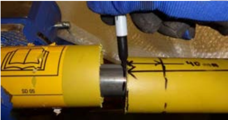
Figure 45 use tube to mark the cut length to steel shaft
