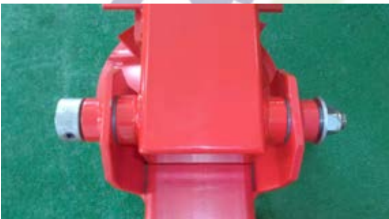
Figure 28 pin is through and the nut is started
