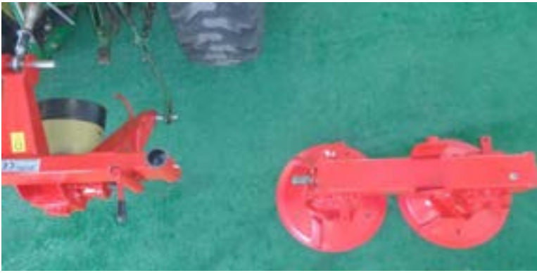
Figure 15 move the drum assembly over to the three point assembly like this
