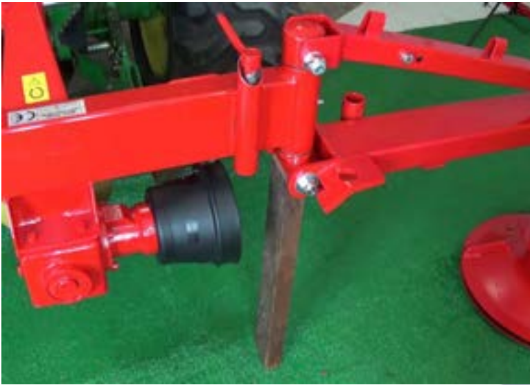
Figure 23 top spring arm installed with pin blocked up by using a 2x4
