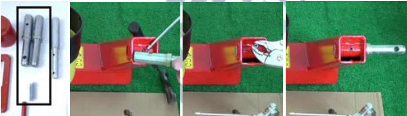
Figure 10 install the pins in the arms as shown on both sides
