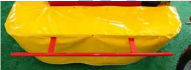
Figure 36 curtain installed with 2 holes for toe guard facing forward
