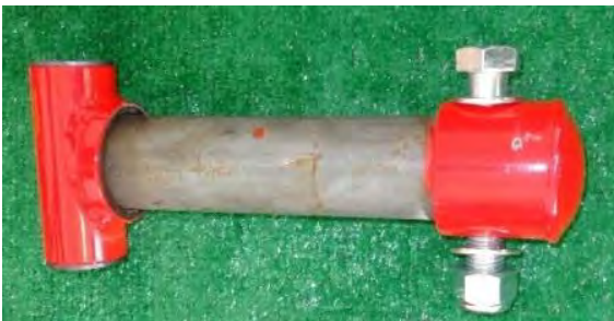
Figure 16 swivel tee identification
