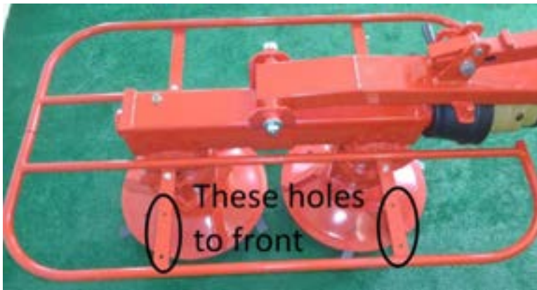
Figure 34 front guard has 6 holes
