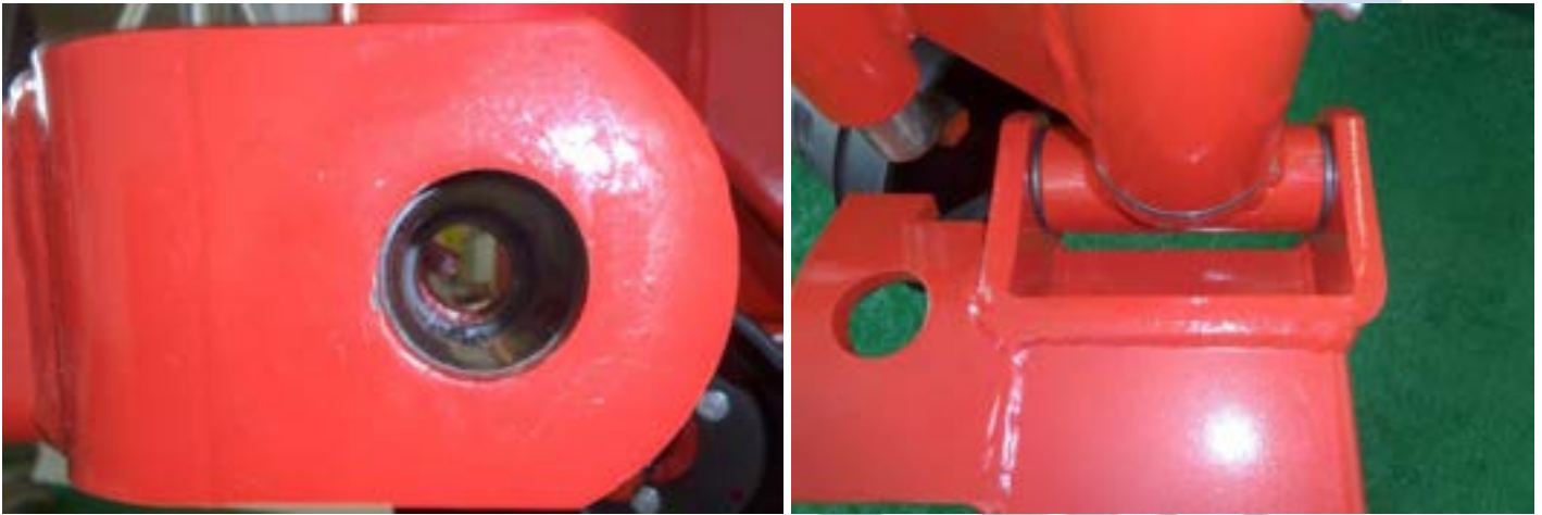
Figure 21 holes aligned to allow pin to pass
