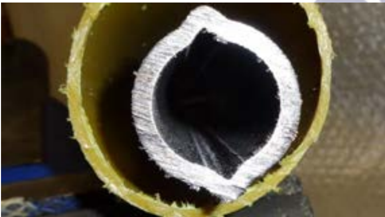
Figure 48 burrs and shavings must be removed
