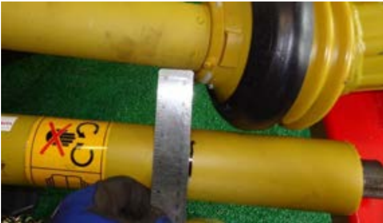
Figure 41 mark overlap length
