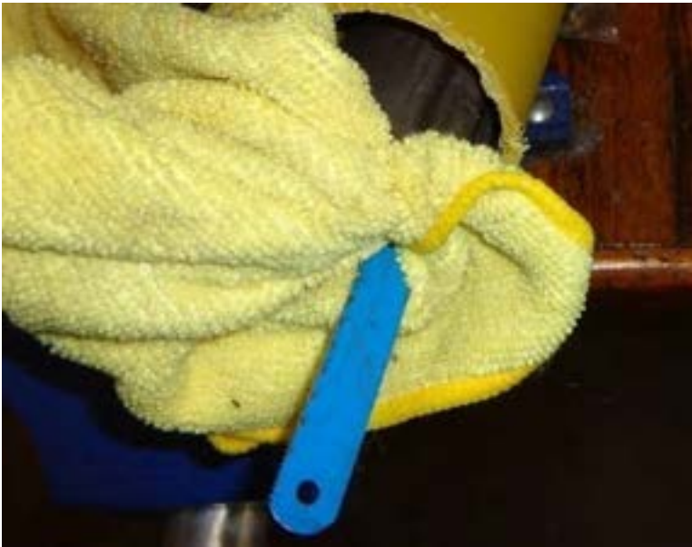
Figure 50 push towel into and around shaft to remove shavings
