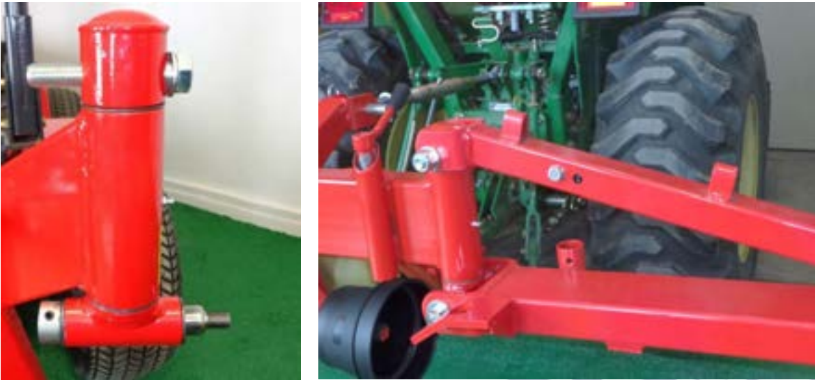
Figure 18 swivel tee in place for next step and the completed assembly to the right
