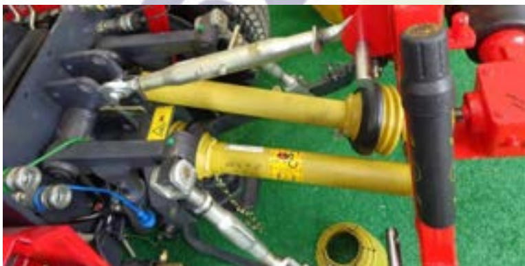
Figure 40 PTO's installed to mark overlap
