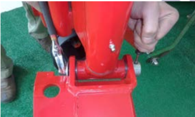
Figure 22 pin through and nut started
