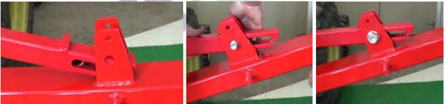
Figure 25 top spring arm attaches to lower arm here
