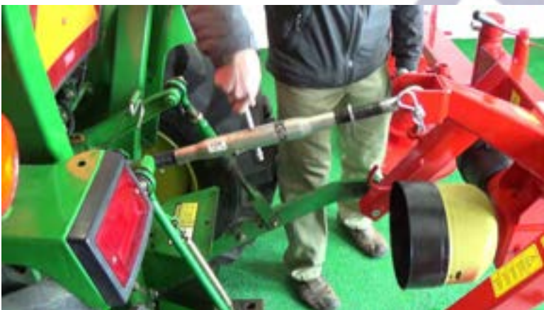
Figure 12 level the 3 point assembly with the top link
