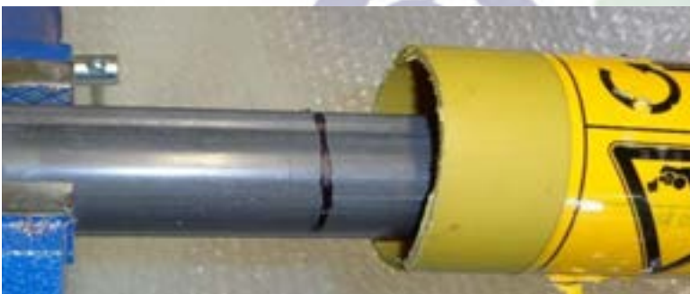
Figure 46 shaft is marked to cut off same length as plastic tube
