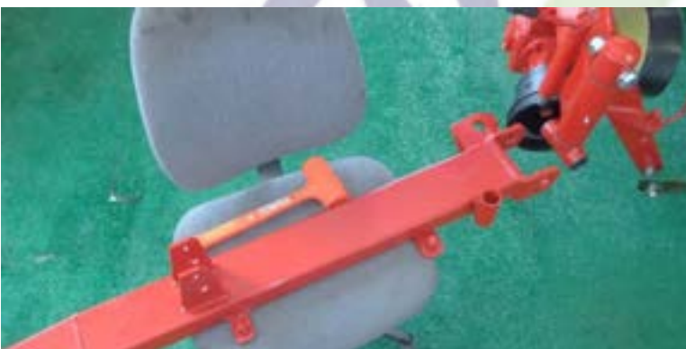
Figure 20 align holes in arm to swivel tee
