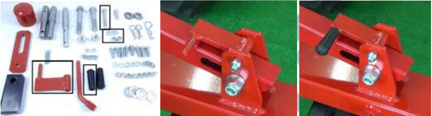
Figure 29 transport lock and rubber grip installation
