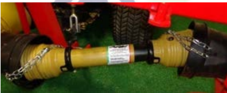
Figure 31 guard chains attached
