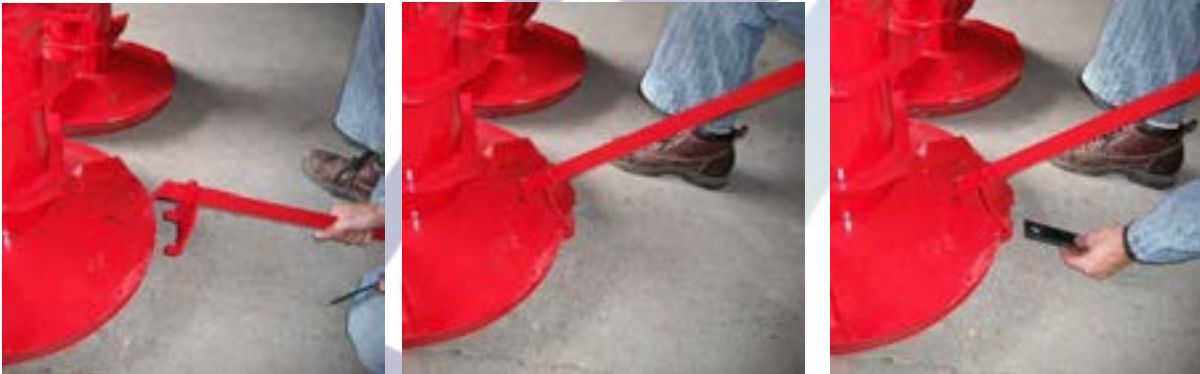
Figure 14 installing a blade.
