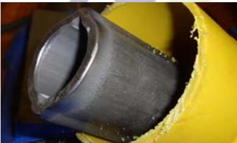
Figure 49 burrs removed with a file, grinder and power wire wheel.
