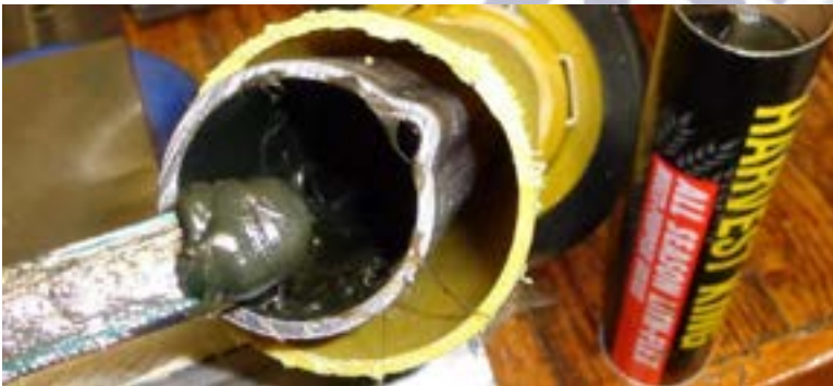
Figure 51 spread grease in outer shaft
