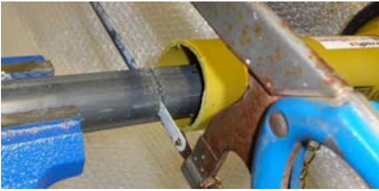
Figure 47 clamp on the part of the shaft that is being cut off then cut
