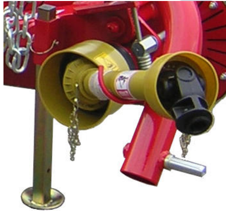
Support leg of the drive shaft
