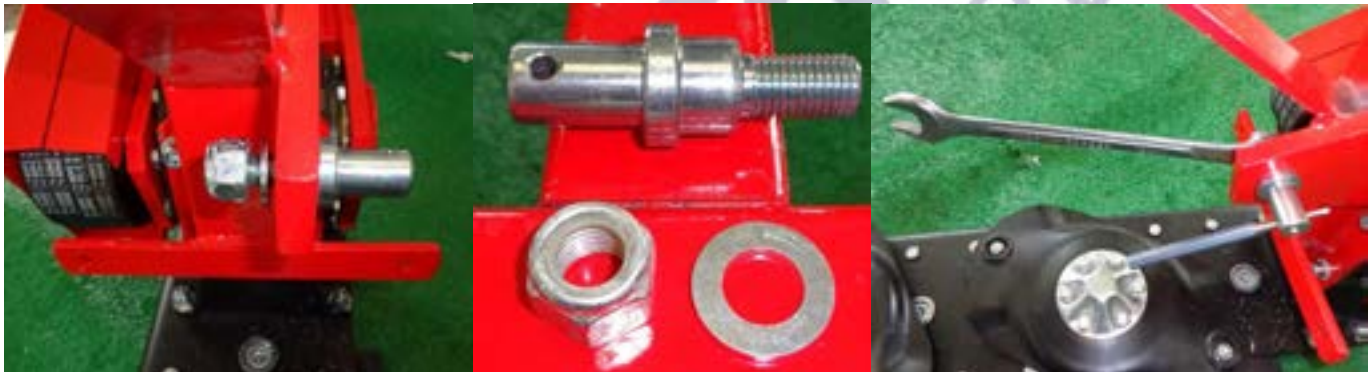
Figure 24 Install pin for telescoping arm through hole as shown
