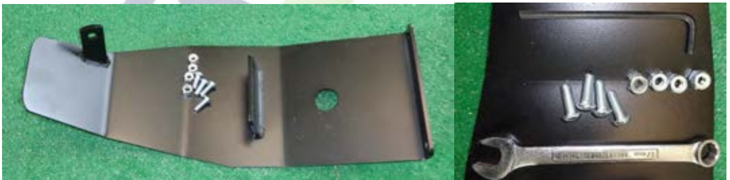
Figure 34 Get the skid plate and the hardware shown and bolt the plate on
