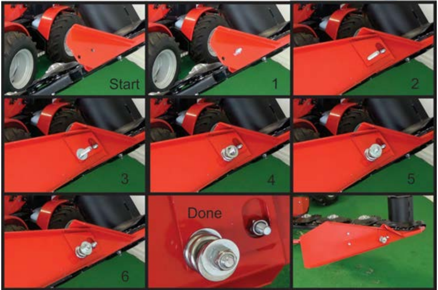
Figure 41 Steps to assemble the outer swath plate
