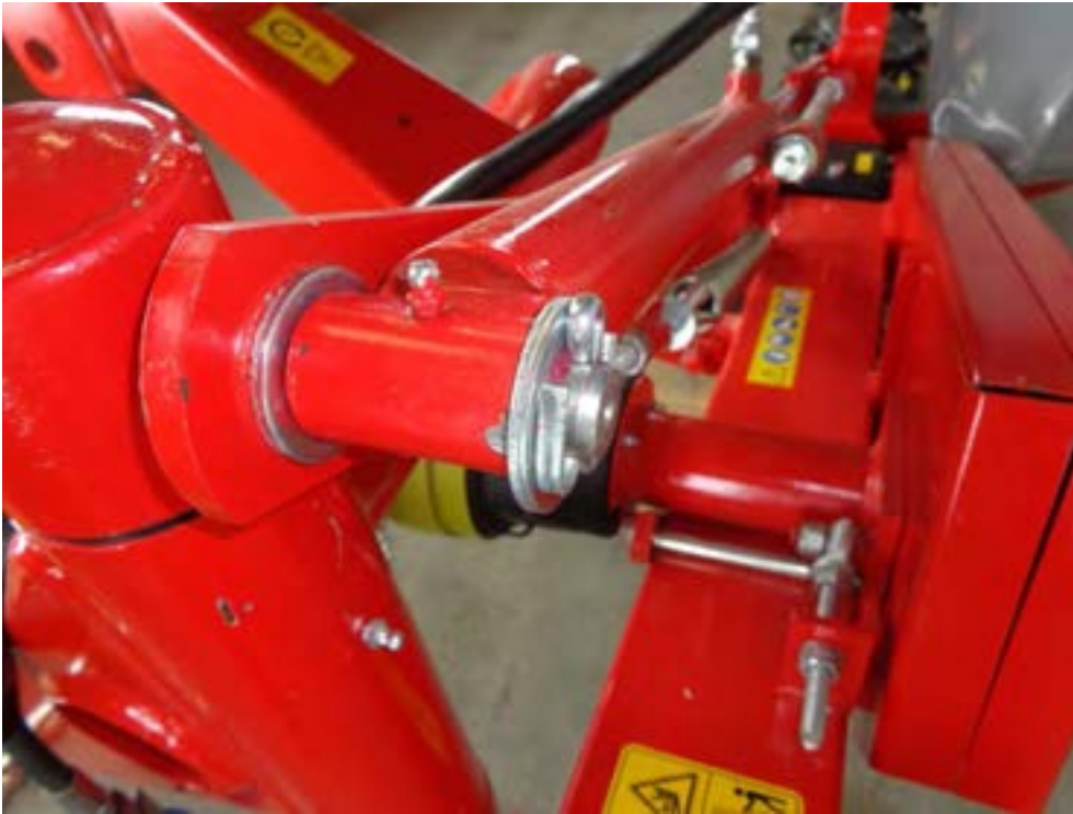
Figure 30 Hydraulic cylinder shown attached to upper pin
