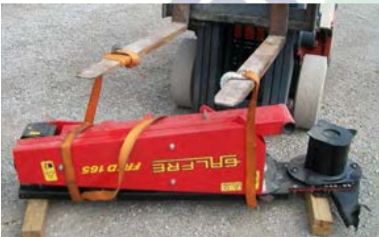
Figure 2 Lifting the disc assembly
