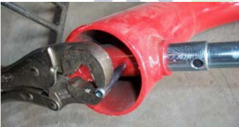
Figure 10 Drive the pin through
