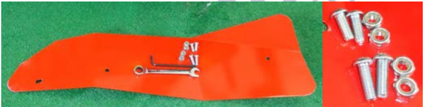
Figure 36 Inner swath plate is attached with 4 cap screws shown
