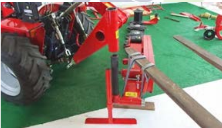
Figure 16 Line up the pin to the hole on the 3 point hitch
