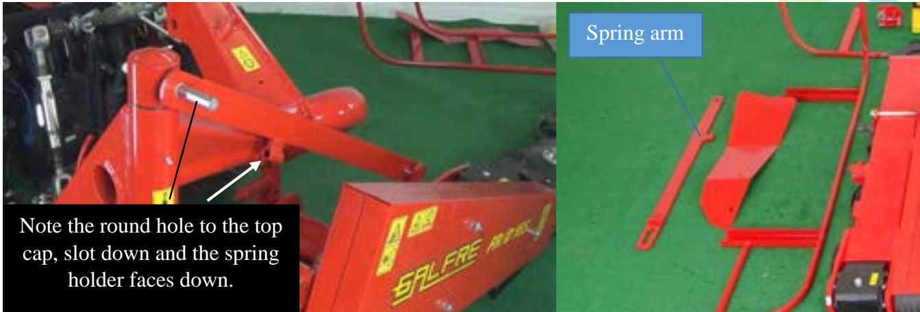
Figure 19 Attaching spring holder arm
