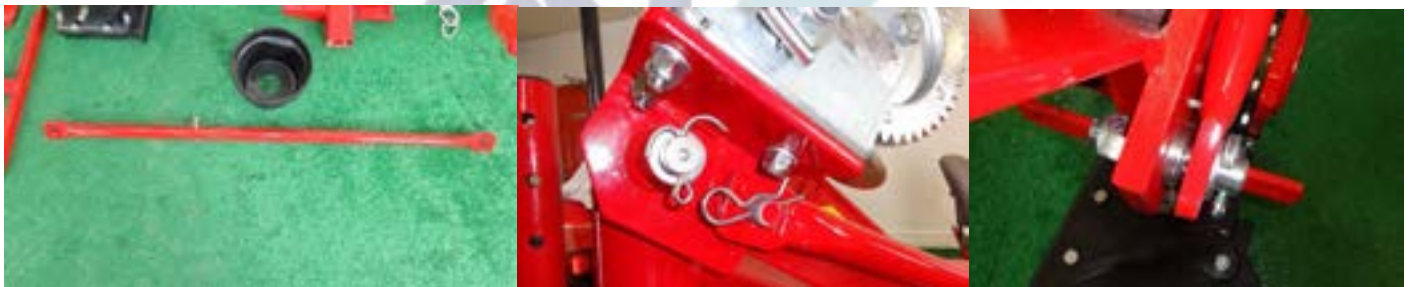
Figure 27 Telescoping arm installs with large diameter tube at winch
