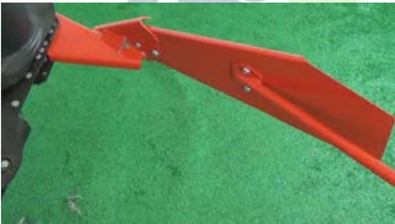
Figure 42 Swath plate rod installed
