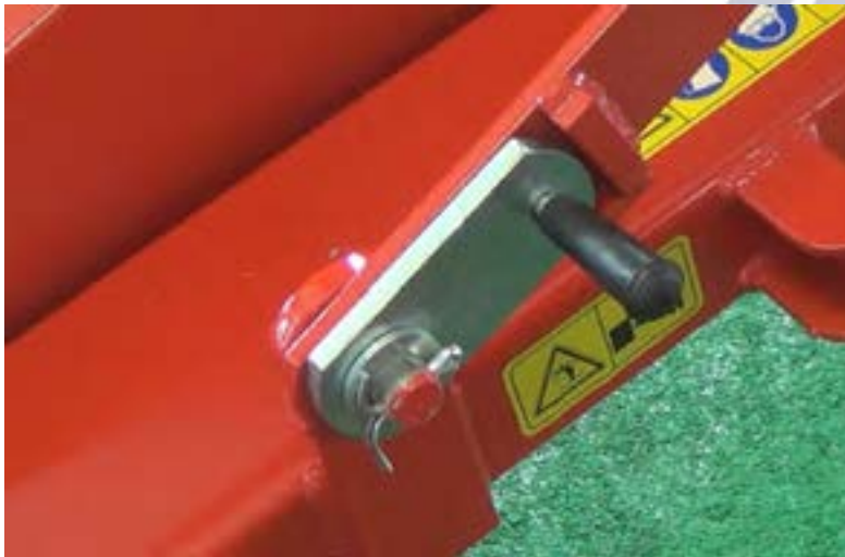
Figure 20 Secure the transport lock
