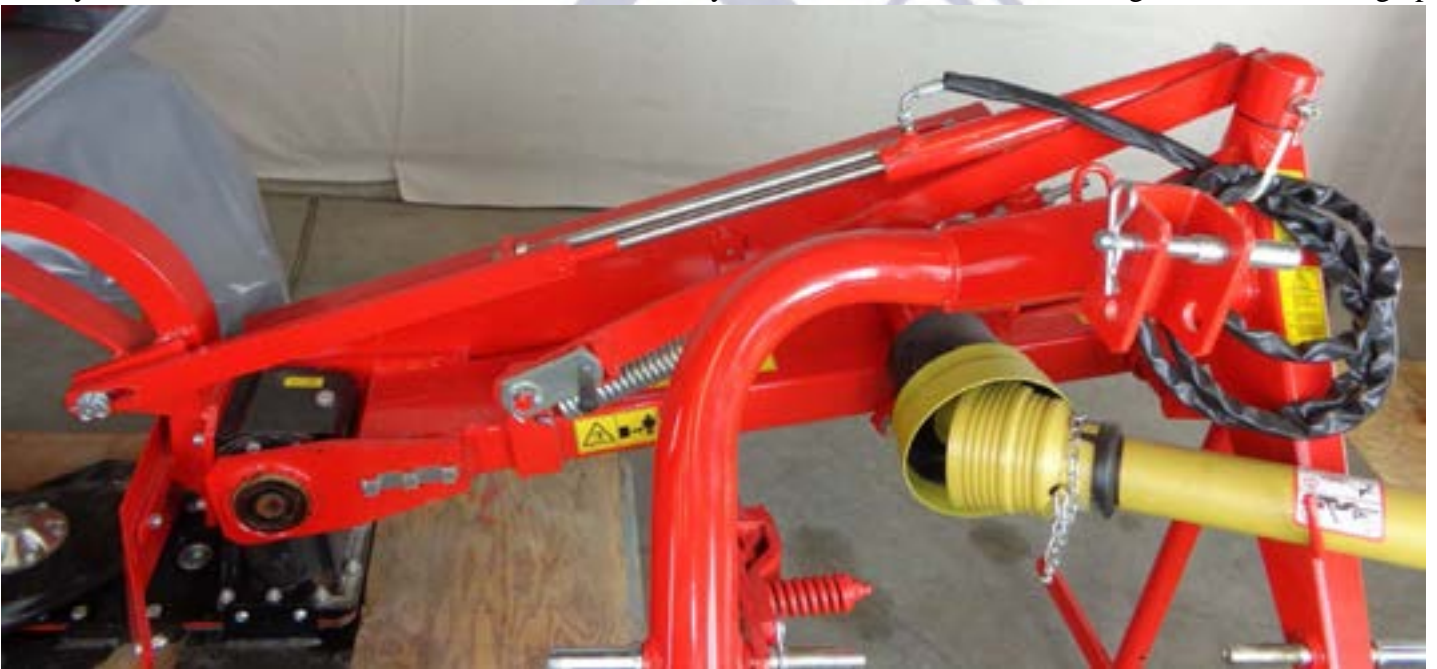
Figure 29 Hydraulic lift cylinder shown installed
