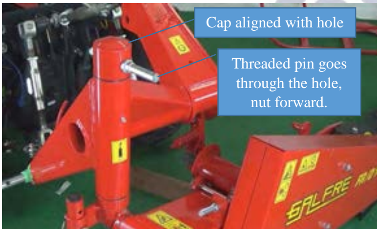
Figure 18 Secure the top cap with pin shown
