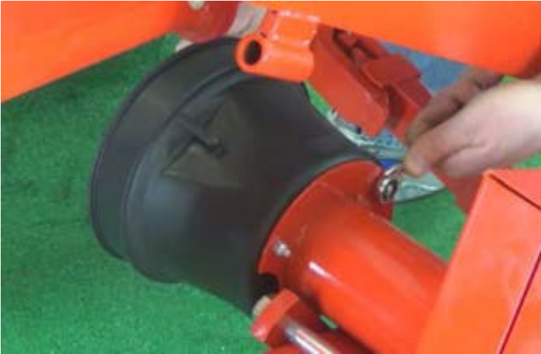
Figure 21 Install plastic PTO driveline shield
