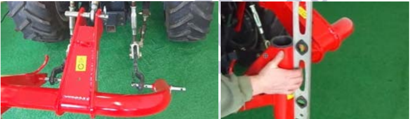
Figure 12 Secure 3 point with top link and level
