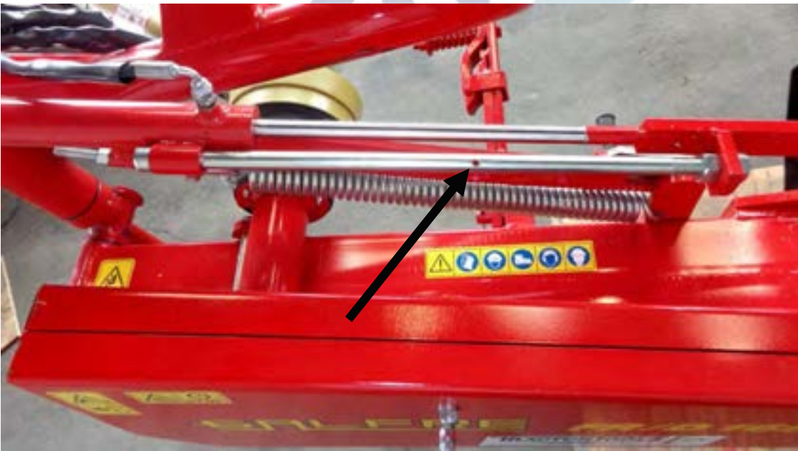
Figure 31 Threaded rod to limit travel and to lock mower up
