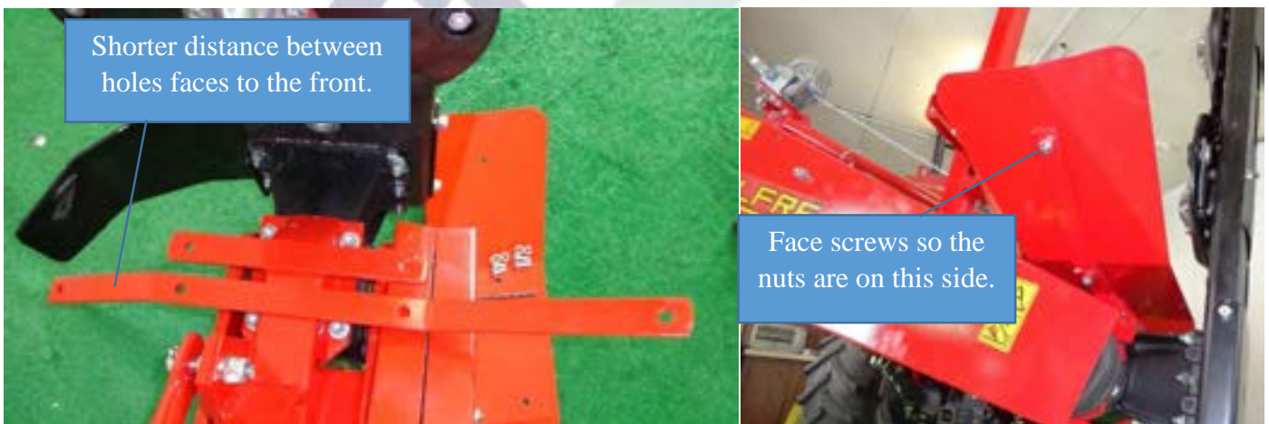
Figure 37 Securing the inner swath plate
