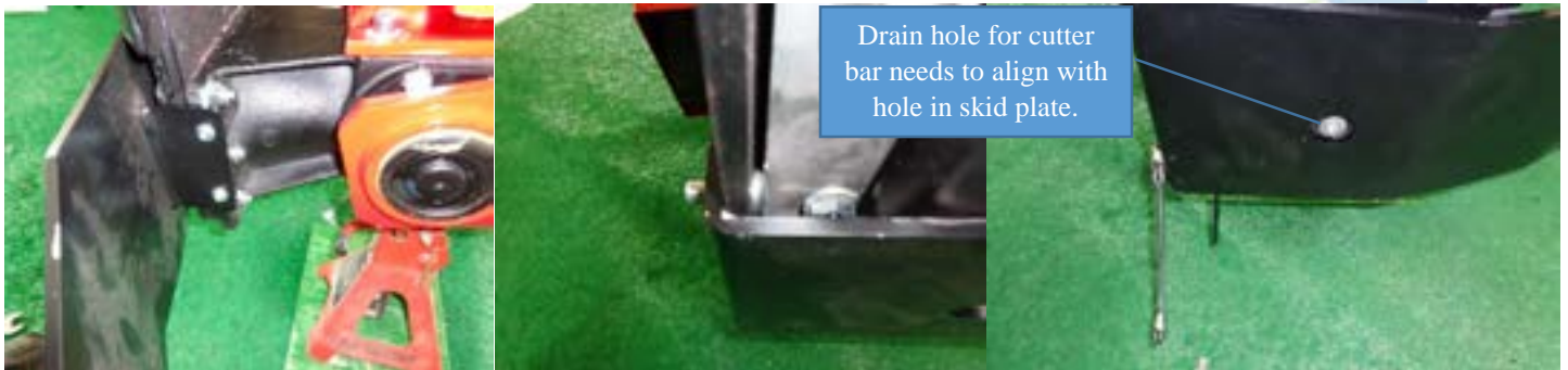
Figure 35 Attaching the skid plate continued
