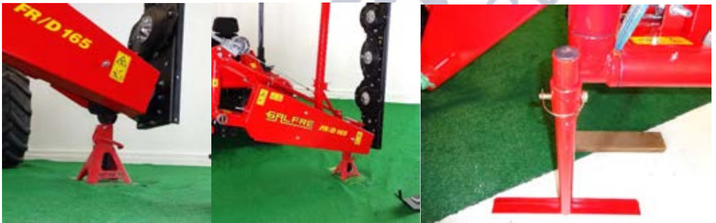
Figure 33 Place a safety stand under the gearbox and lower the jack stand
