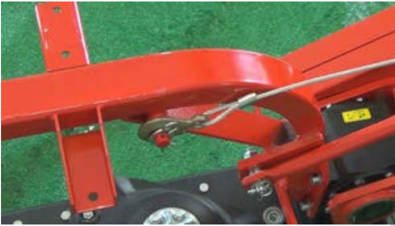
Figure 28 Winch cable attachment point
