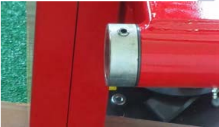
Figure 15 Collar ring secured to swivel pin with roll pin
