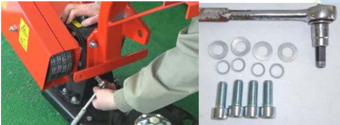
Figure 23 Attach the upper frame to the gearbox
