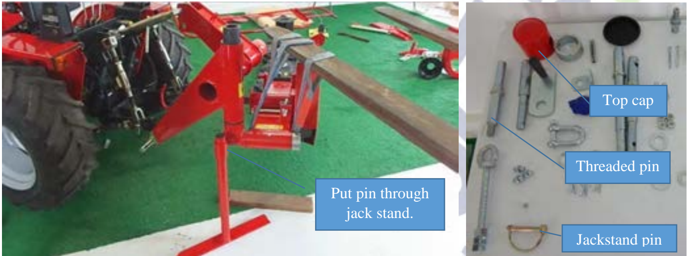
Figure 17 Swivel pin is through the 3 point hitch
