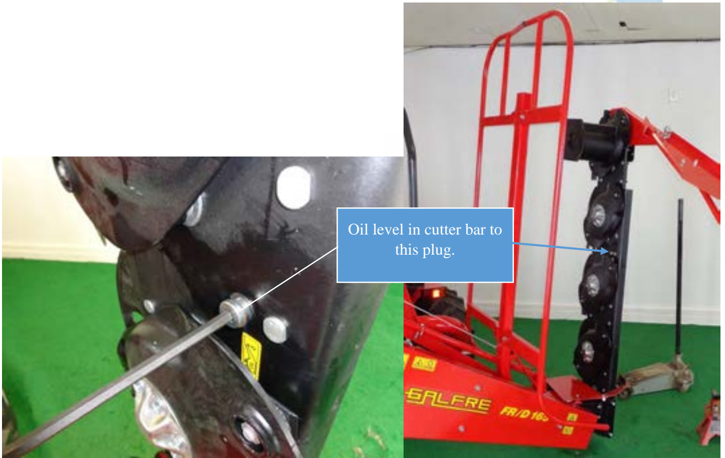
Figure 44 Oil level and fill hole for cutter bar
