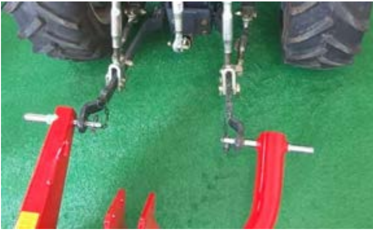
Figure 11 Attach the 3 point frame to your tractor
