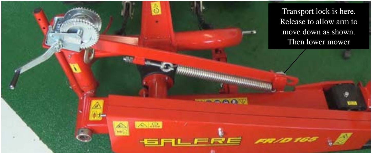
Figure 26 Lower 3 point hitch and attach the spring
