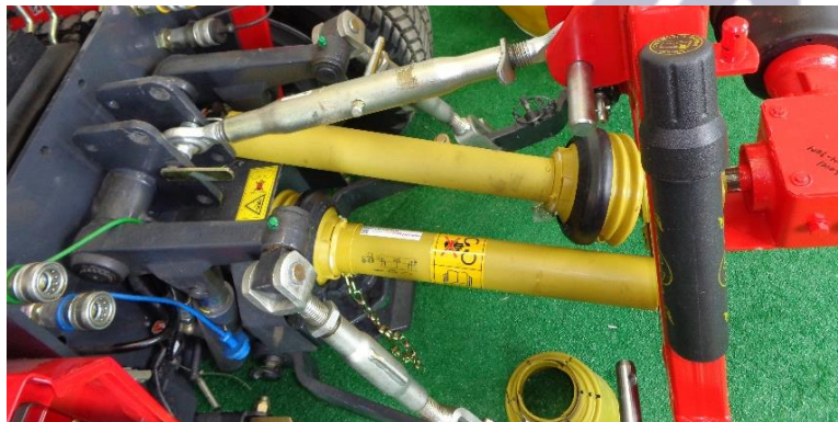
Figure 36 PTO's installed to mark overlap
