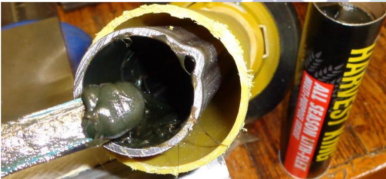
Figure 47 spread grease in outer shaft
