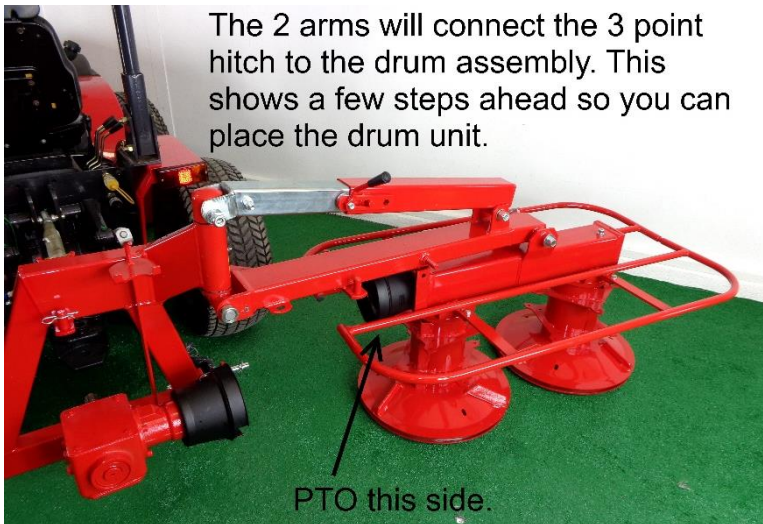
Figure 15 move the drum assembly over to the three point assembly like this
