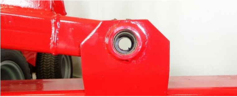
Figure 28 holes are close to being aligned
