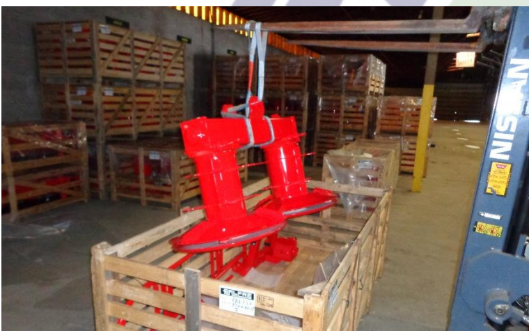
Figure 2 lifting the drum assembly
