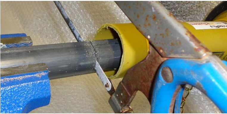
Figure 43 clamp on the part of the shaft that is being cut off then cut
