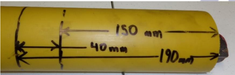
Figure 38 cut off length marked
