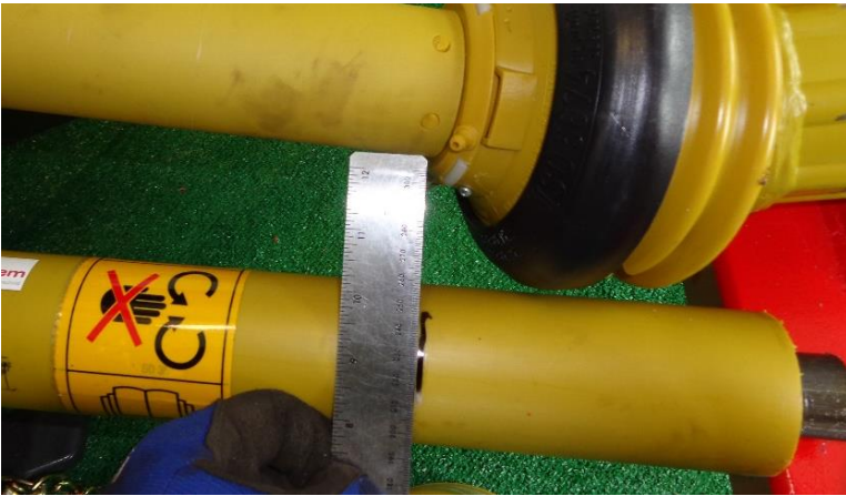
Figure 37 mark overlap length
