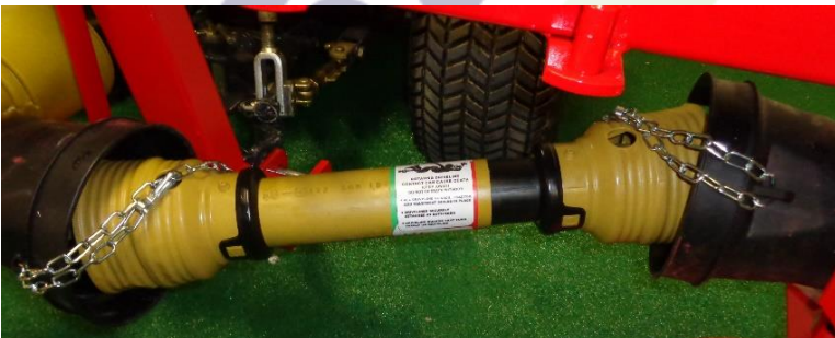
Figure 30 guard chains attached to keep PTO shields from spinning
