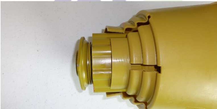
Figure 50 the split end of the guard will fit over the clutch end of the PTO shaft
