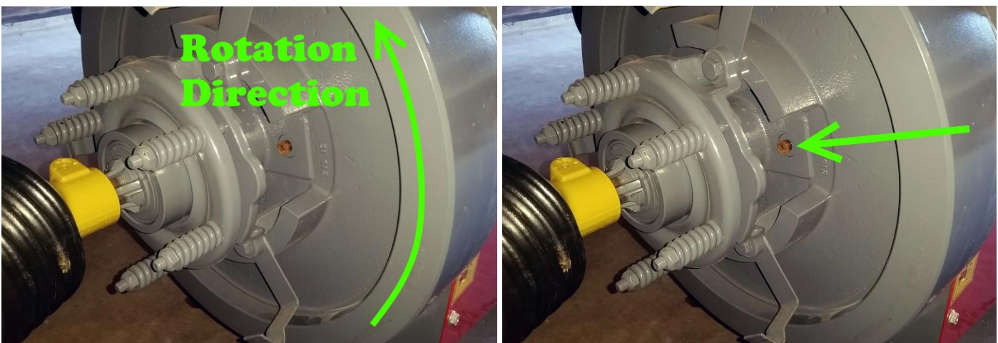
Figure 2 rotation direction and shear pin location on front of flywheel
