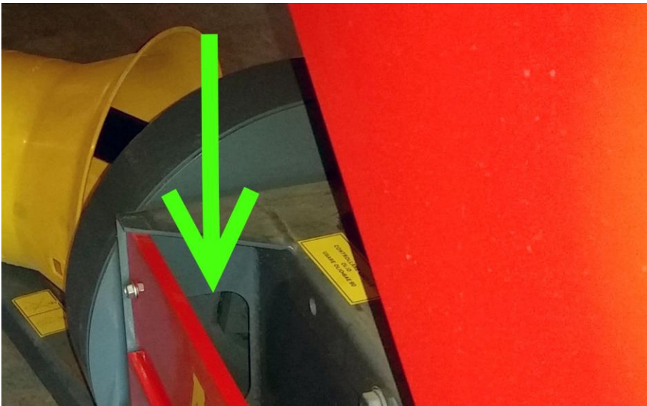
Figure 1 access hole behind the flywheel
