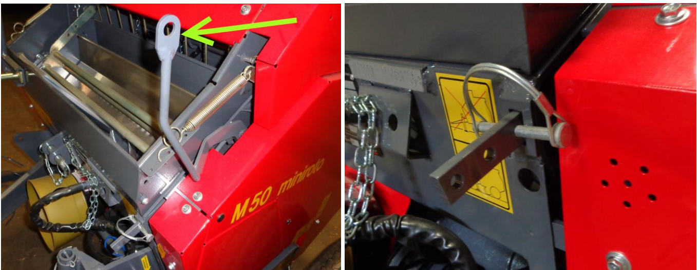
Figure 19 pickup height handle and pin shown in transport position
