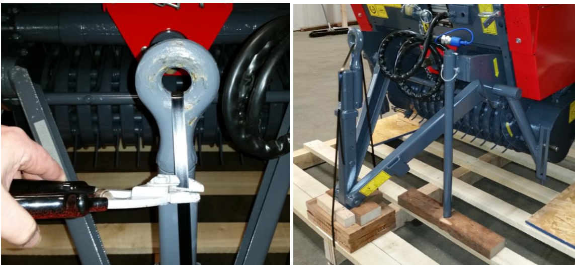
Figure 5 cut steel strap holding the draw bar down
