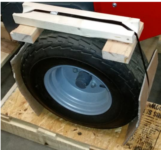
Figure 3 leave the steel strapping in place
