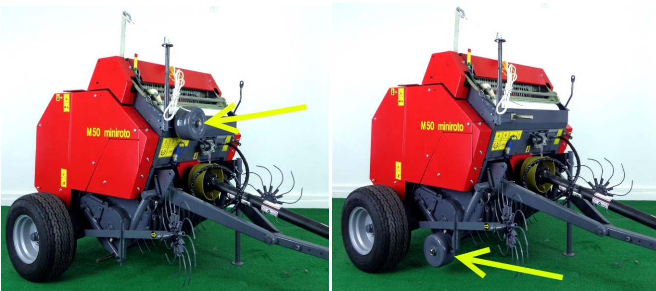
Figure 21 gauge wheel shown in stored position and the bale position
