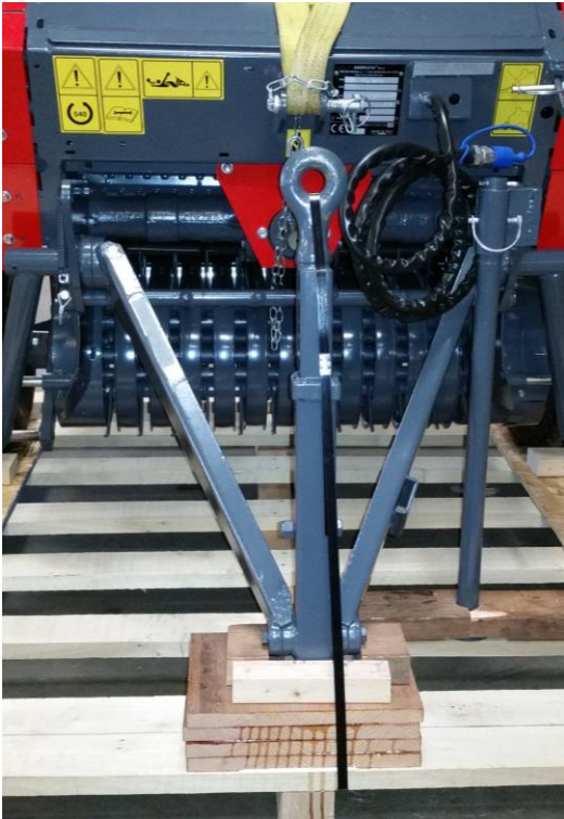
Figure 2 center draw type are attached to the pallet with the draw bar folded up for shipping
