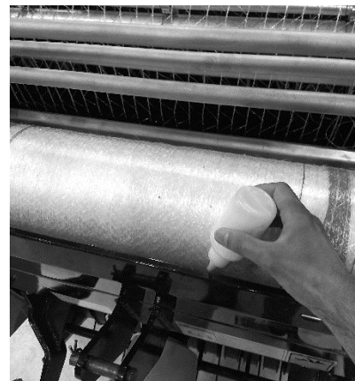
Figure 27 Applying talc powder to front of net roll
